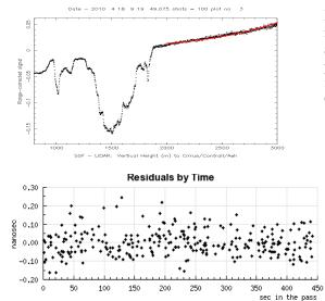
Making some assumptions about the characteristics of the ash (e.g., that its mass attenuation coefficient is about 0.6 m<sup>2</sup> g<sup>-1</sup>), we use the observed attenuation and physical depth of the plume to infer a concentration of the ash particles of about 150 micro-grams per cubic m. A full analysis of this data set is underway in collaboration with Cambridge University and the UK Met Office.
