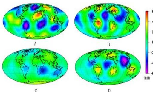
**Annual variation in the geoid for a 6x6 field; (A) cosine and (B) sine component from SLR +CHAMP; (C) and (D) from model GPH4.**
