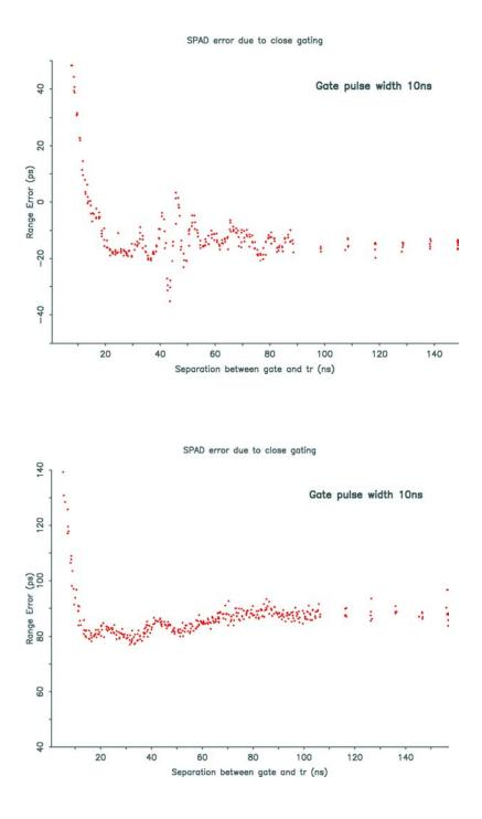
There is a clear improvement in the SPAD detector profiles from the older C-SPAD to the new SPAD, with a much smoother, and therefore predictable, range error which can be removed from real data. However the new SPAD profile still contains two small error 'peaks' at 20ns and 40ns, meaning that the minimum safe gate will be at about 50ns.
