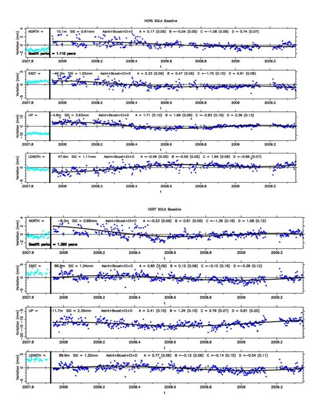
The GPS analysis also takes a global network of GPS sites and uses the GAMIT/GLOBK software along with downloaded IGS orbits and EOPs, to produce daily and weekly coordinates for the HERS and HERT sites. These include an 'UP' component for comparison with SLR analysis, absolute gravimetry and water table heights.
