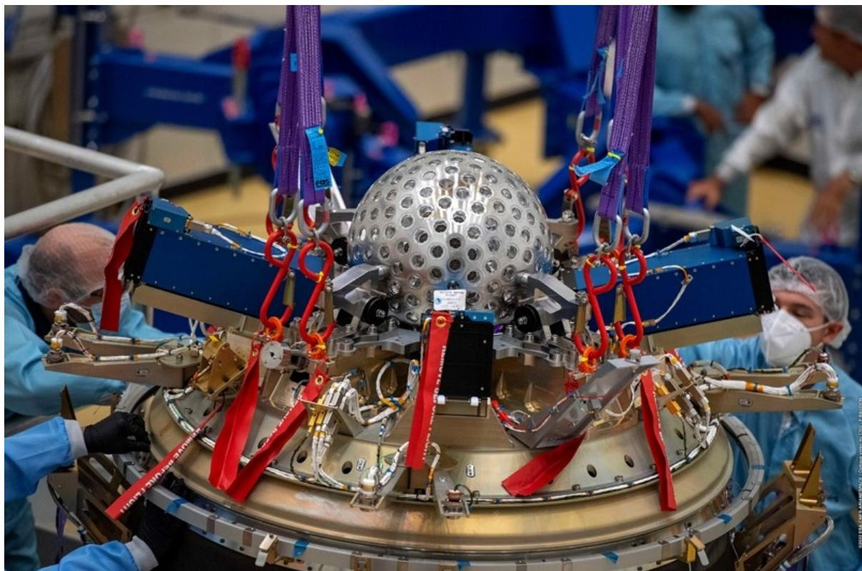
Figure 1: Installation of LARES-2 into the Vega C launcher. The surface of the satellite is covered in 303 reflectors that will reflect laser pulses sent out by a global network of laser-ranging stations. Credit: CNES/ESA/Arianespace/Optique Vidéo CSG/P. Baudon
